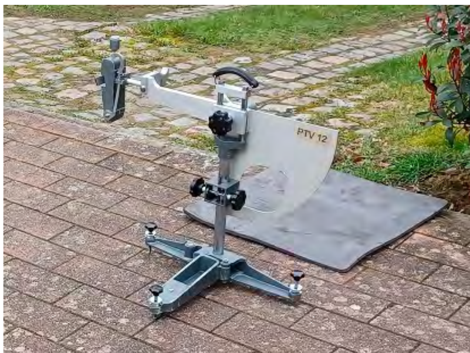
Figure 1 - Le pendule SRT © CRR
