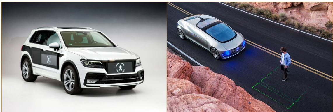
Figure 5.10 – Example of a vehicle with multiple information screens for communication with pedestrians (Volkswagen Tiguan) – projection of road crossing (Duff, 2015; Light staging and exterior HMI, 2018)
