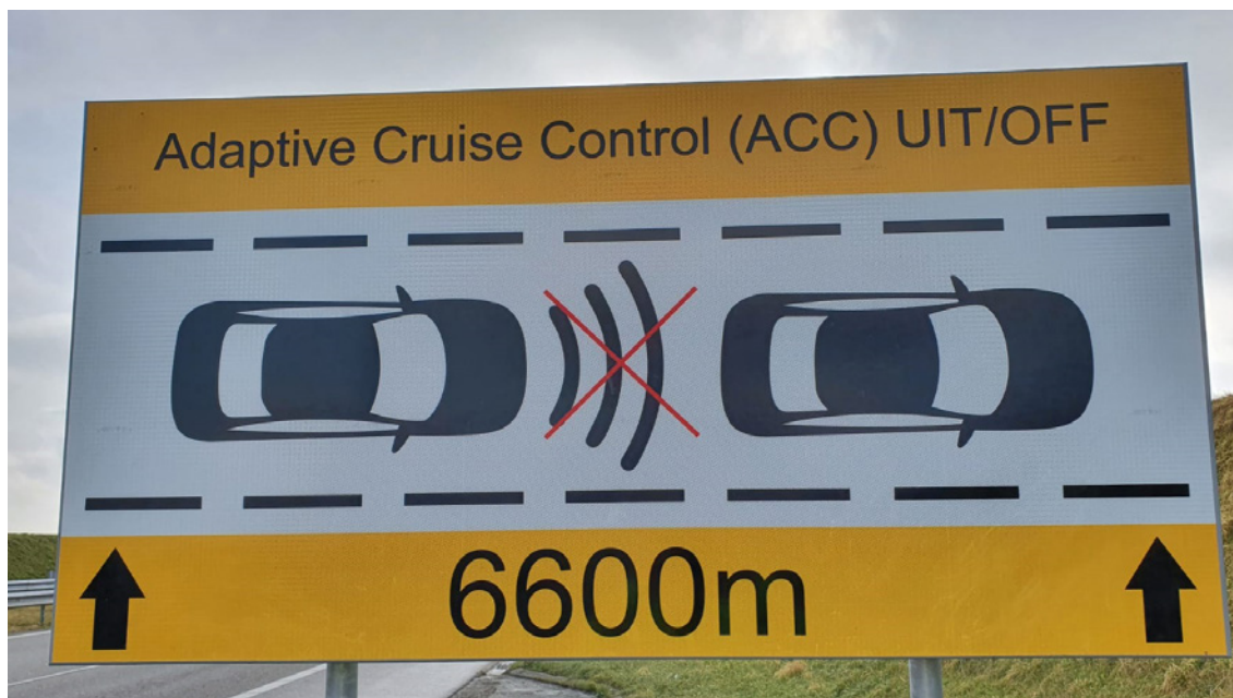
Figure 2.7 – Traffic sign recommending disabling ACC (Western Scheldt Tunnel, Netherlands (Adaptive cruise control, 2021)
