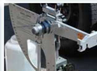
Skid Resistance Tester (SRT)
